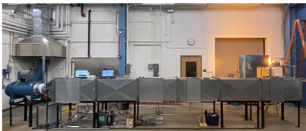
Figure 2: Photo of the Purdue University HVAC filter test rig.
